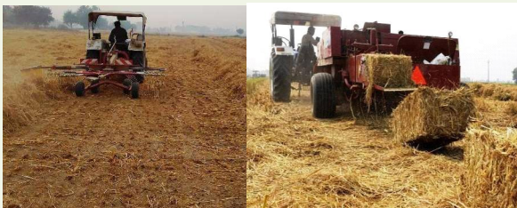
Rake and baler machine in operation
